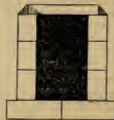
Fig. 5.—SECTION OF FLUE.
