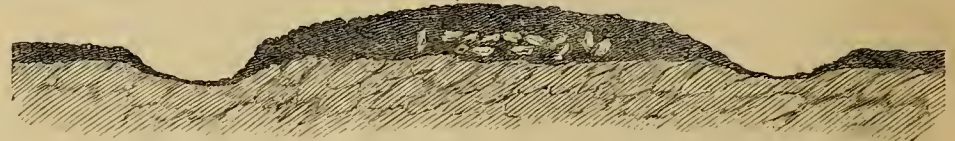
Fig. 2.—THE ROAD "MADE"—ALL THE SURFACE SOIL OF THE GUTTERS BEING PILED ON IT.
