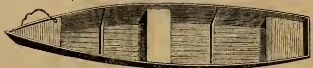
Fig. 5.—BOAT, SHOWING RIBS, LOCKERS, AND SEAT.
