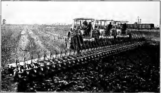
FIG. 5. The "Oil Pull" Gang Plow which, in a demonstration in 1911, with three engines, did the work of 100 men, 200 horses, and 50 plows, plowing 14 acres an hour at a fuel cost of 6½ cents per acre.
