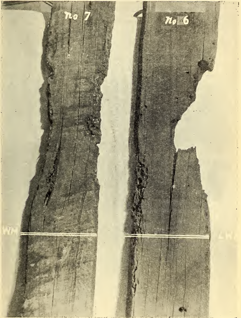
Longitudinal Sections of two Piles showing ravages of Limnoria and Sphaeroma . The right hand side of No. 6 is the work of the Limnoria ; the remainder Sphaeroma . There are very few Cobra holes.
