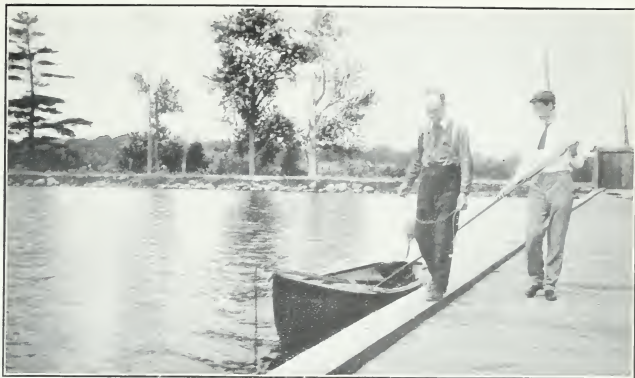
No. 11.—Rating meter at Dow's Lake, Rideau Canal. Boat being towed at a slow speed. For this rating speeds varied from .96 ft. per sec. to .9 ft.
