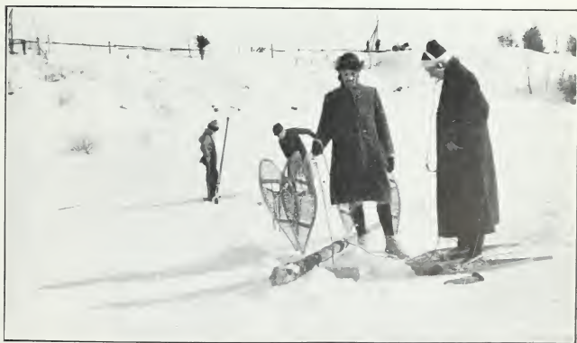
No. 40.—Current meter is in the water. Engineer is timing the revolutions of the wheel by means of a stop watch and telephone receiver.
