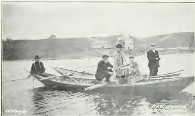
No. 14.—Photograph showing method of metering where channel is sufficiently narrow to allow of a rope and cable being stretched.
