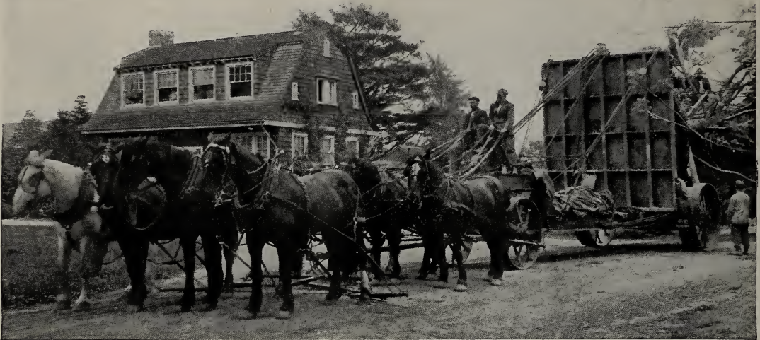
Tree-Mover No. 21. Moves evergreens and other trees with very large balls of earth. This is one of two Pines moved from our nursery to the church half a mile east. The big steel platform and frame are worth seeing
