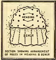
HEADING- AND BENCH-DRILLS AT WORK.
