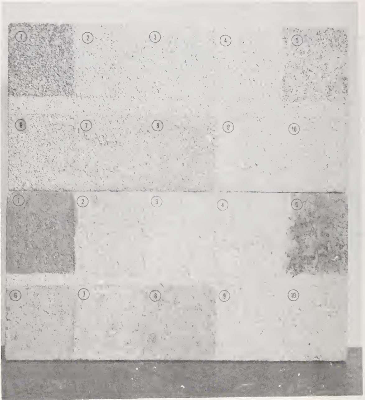
Figure 6. Masonry units illustrating changes in appearance caused by waterproofing materials Nos. 1-10. The upper unit is a lightweight aggregate block while the lower unit is a dense aggregate block. The horizontal strip across the middle of each block is an uncoated area for comparison.
