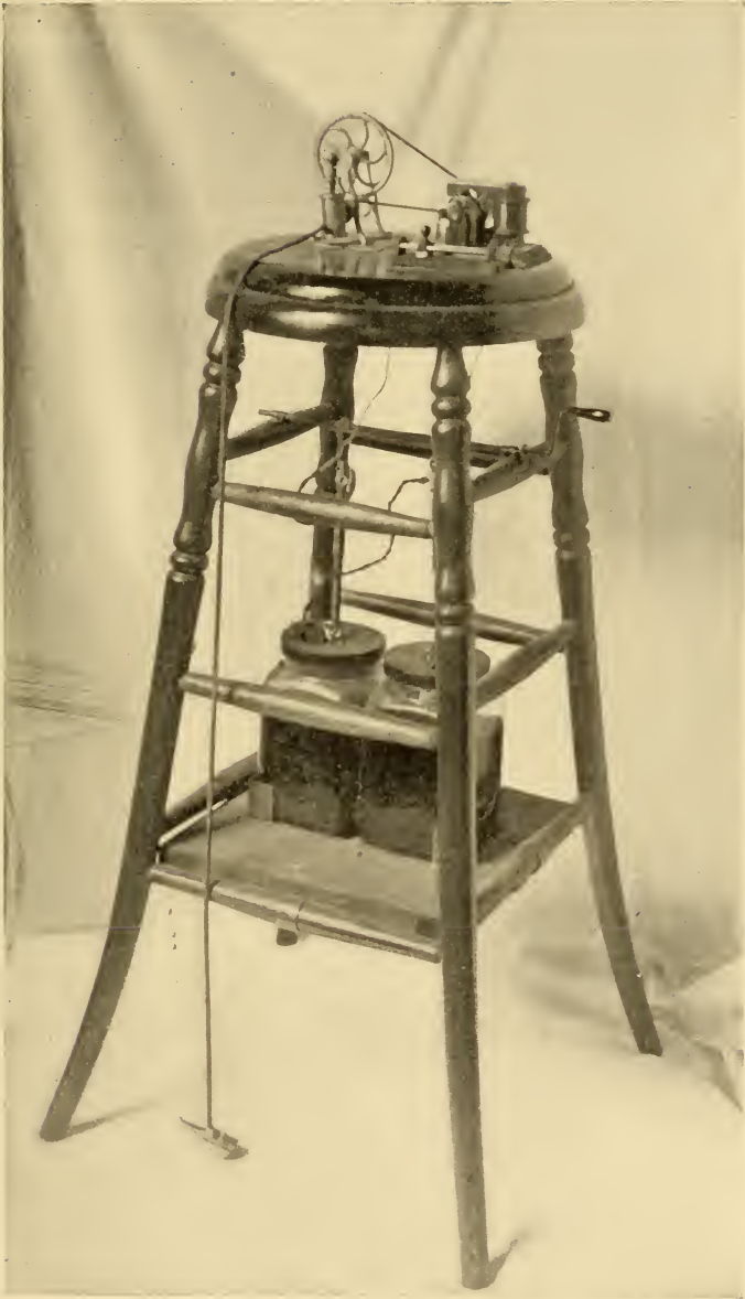
Burnett's mounting of the Chevalier Jackson pneumatic masseur, fitted with the modified Siegle pneumatic otoscope.
