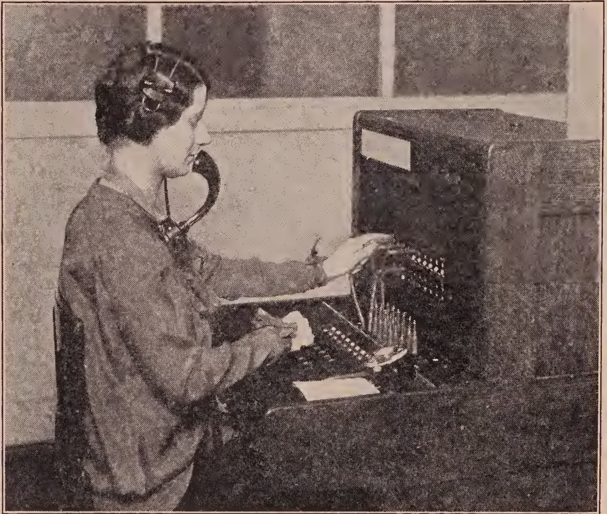
One-position Private Branch Exchange of the Cord Type, with Dial
