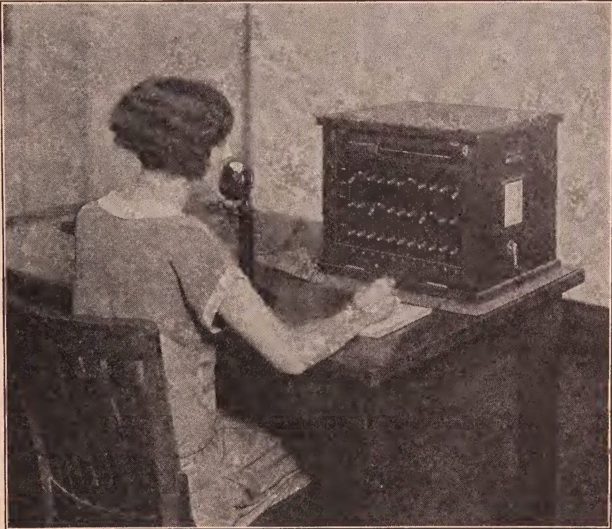
Small Cordless or Monitor Switchboard, Operated by Keys
