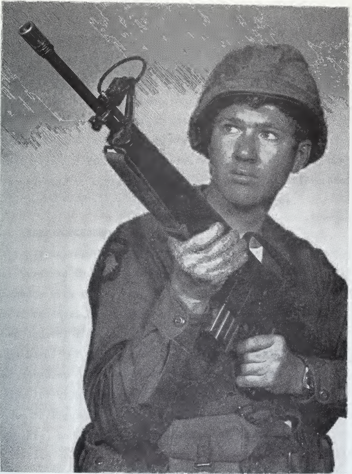
Figure 7. Infantryman at the Ready Holding M16A1 Rifle with 2.64" dia Experimental Bracketing Sight.
