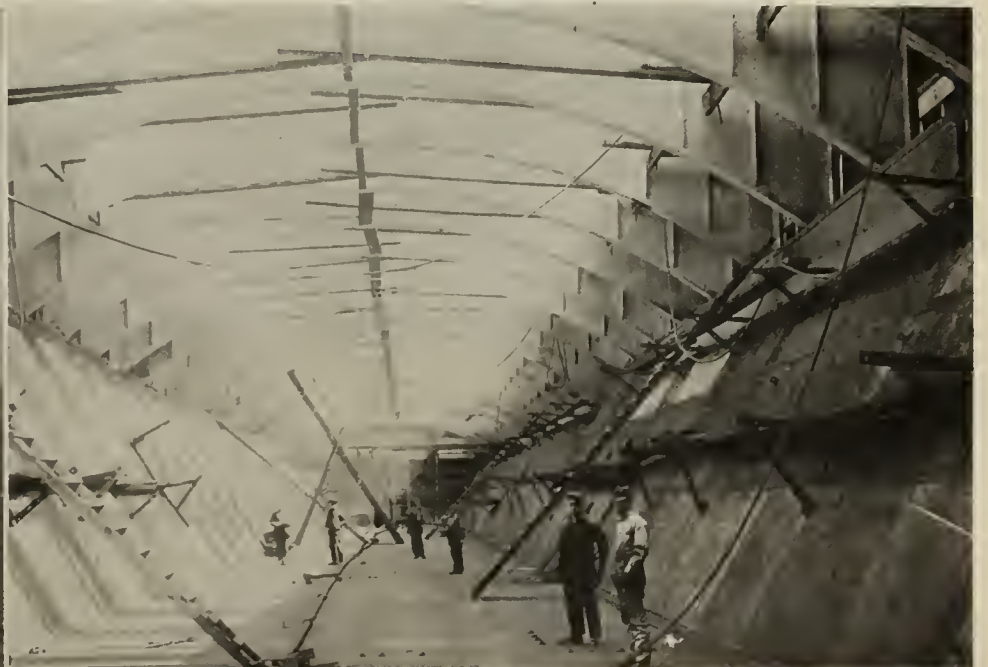
Interior of a Great Lakes Grain Carrier in Process of Construction, Showing the Capacious Hold.
