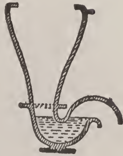
Figure 38. The hopper closet.
