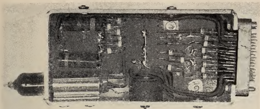
Packaged circuitry of this type (actual size shown) is expected to simplify construction and maintenance of electronic computers (p. 96).
