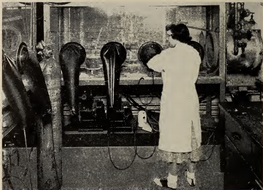
Inert atmosphere chamber used in studying electrodeposition of metals from nonaqueous media. The chamber permits filtration, distillation, transfer, and weighing of reactants or products without contamination from water or carbon dioxide.
