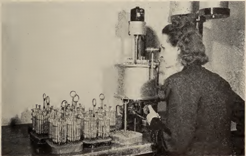
Diagram illustrates how the international temperature scale maintained by the Bureau is translated into practical use for the benefit of science, industry, and the public. Photograph shows thermometers are being calibrated against a "standard" liquid-in-glass thermometer. During 1955 the Bureau calibrated over 33,000 clinical thermometers.
