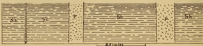
Fig. 5 Vertical section of Clintonville dikes, March 23, 1910 Sh = shale P = peridotite dike
