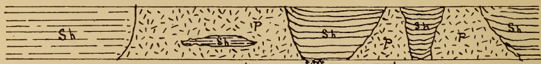
Fig. 4 Section of Green street dike along excavation made by electric light company, November 24, 1905. Sh = shale P = peridotite
