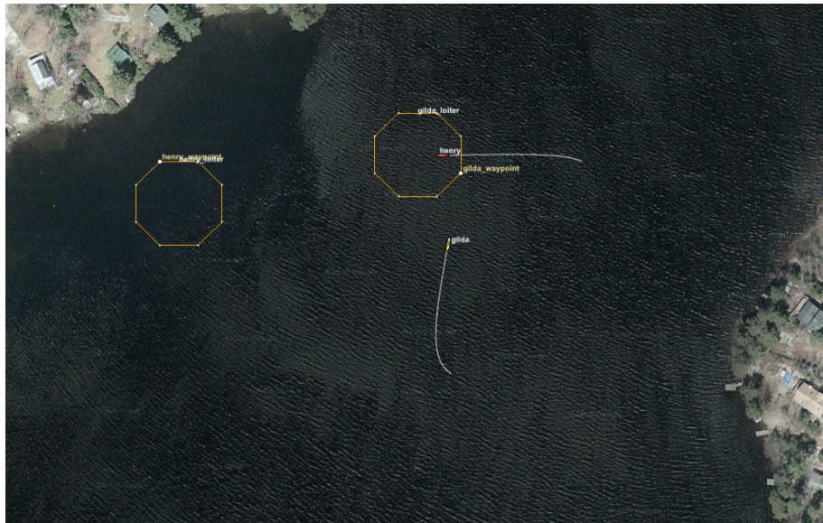
Figure 3-11: Two vehicles alternated between North-South and East-West polygons. These polygon positions were randomly positioned ensuring that each permutation resulted in a new geometry and timing. The results were then examined in detail including the criteria that triggered entering and exiting the collision avoidance rules. This test proved invaluable for refining the entry and exit criteria for stand on and give way rules. This image shows vehicles transiting to polygons in north and west zones.
