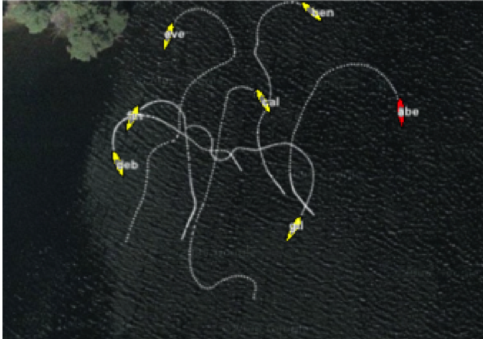
Figure 3-12: A swarm of seven autonomous marine vehicles was allowed to operate toward randomly generated points in a high contact density environment. The vehicles were maintaining collision avoidance in accordance with COLREGS and finally ordered to seek a convoy pattern to the south while maintaining collision avoidance.
