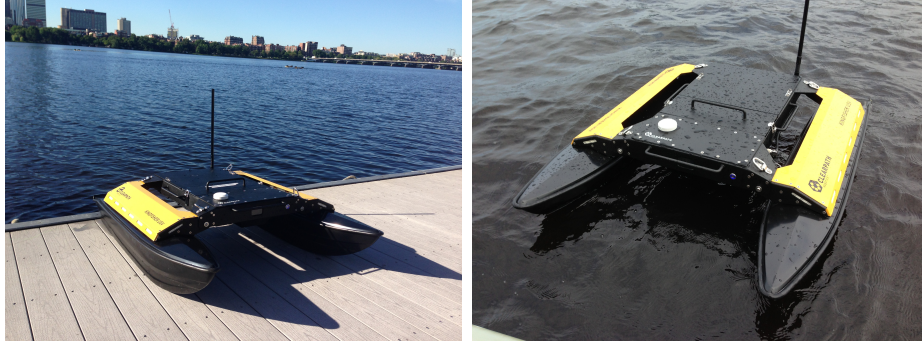
Figure 2-4: The Clearpath M200 autonomous marine vehicle is a catamaran, water jet driven design used for testing on the Charles River.
