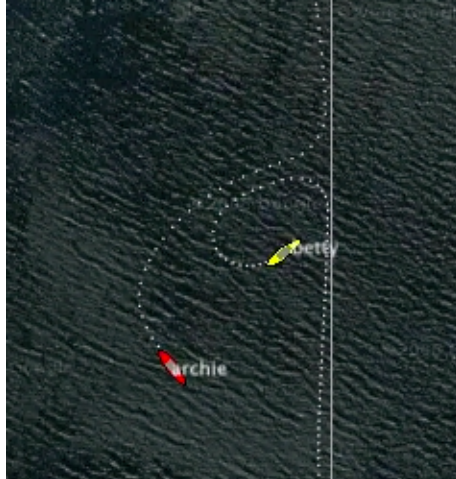
Figure 3-1: In this example, an AMV deviates from course much more than necessary to avoid a collision due to an inefficient and unsafe symmetric maneuver by the second AMV.
