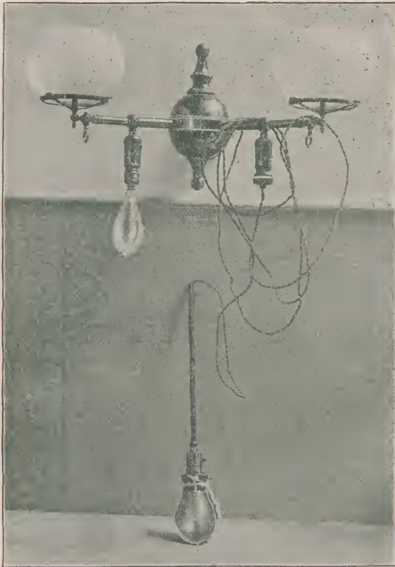
FIG. 2.—Electric drop-light for use in abdominal operations, connected with house circuit.
