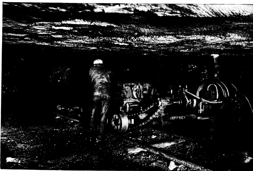
ELECTRIC CONTINUOUS CUTTER MOUNTED ON TRUCK, READY FOR OPERATION
