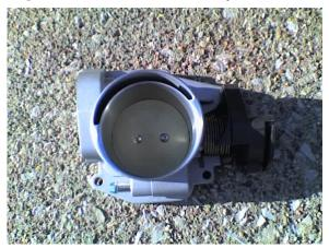
Figure 9 The Fastman Throttle Body
