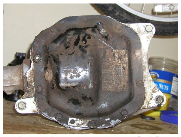
Figure 10 2005 Jeep Liberty Dana 30a Front Axle Housing and Differential Cover
