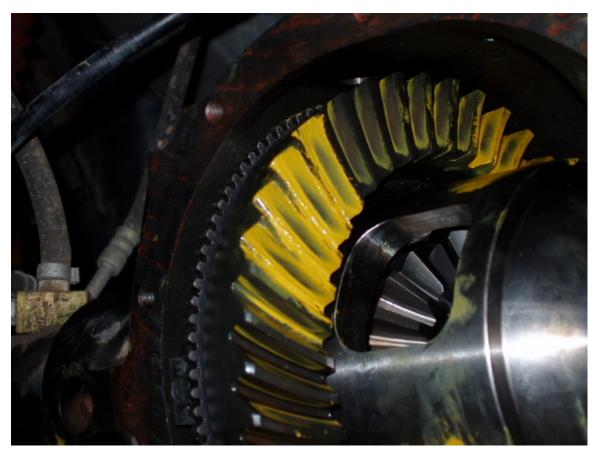
${\bf Figure~14}~~{\rm Yukon~4.10~Chrysler~8.25"~Ring~\&~Pinion~Drive~Pattern}$
