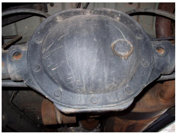
Figure 11 2005 Jeep Liberty Chrysler 8.25" Rear Axle Housing and Differential Cover
