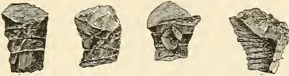
Fig. 130.—Deformation of leaden bullets (natural size) (Seydel).
