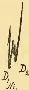
FIG. 5. A bolograph of the sodium double yellow line indicating the nickel line between them. This will show the extreme delicacy of this method of feeling and recording absorption lines.
