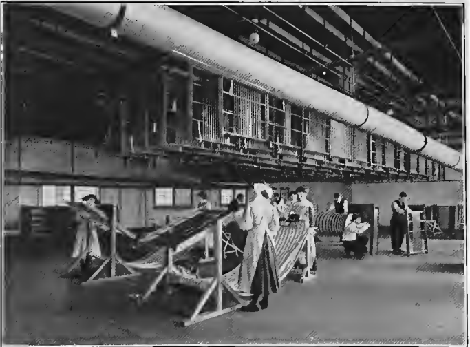
Film-Drying Room in a Film Factory. The Films are Rolled Around and in the Air
