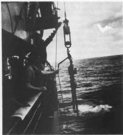
DEEP SEA DIGGING—Dr. Harris B. Stewart, Oceanographer, U.S. Coast and Geodetic Survey, pulls release pin from a Phleger corer to drop it 2 miles from the ship "Explorer" to the ocean floor. The 4-foot core bored from the ocean bed will be studied by Federal geological oceanographers to learn more about the history of the sea and the land beneath. Many scientists believe that oceanography will contribute much to the future of mankind. (Official Coast and Geodetic Survey Photo)
