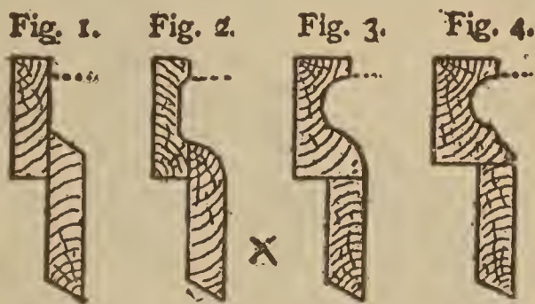
SECTIONS OF NOSING MOULDS WITH RISER BOARDS.
