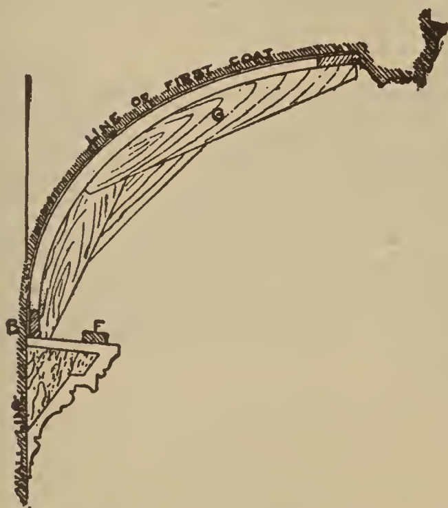
SECTION OF COVE SHOWING PRESSED SCREED PROCESS.
