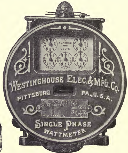
FIG. 239.—Two-wire Single-phase Integrating Wattmeter.
