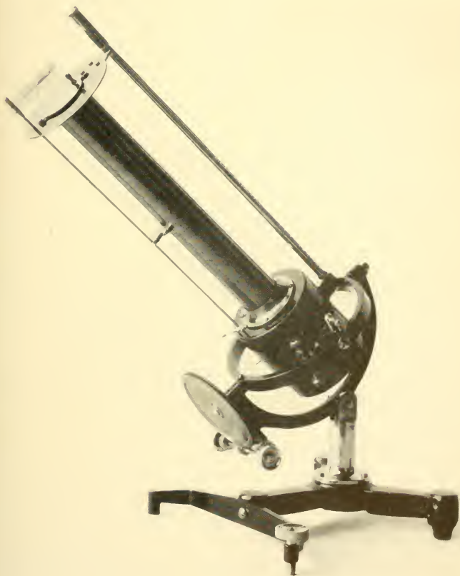
ABBOT SILVER-DISK PYRHELIOMETER, WITH LONG TUBE ADOPTED 1927
