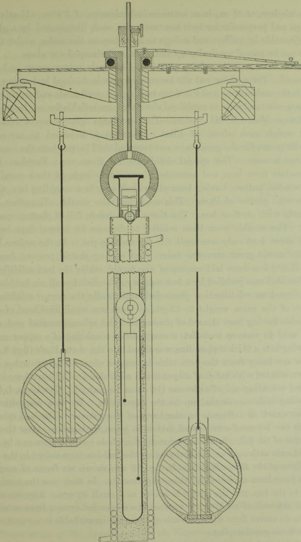
Fig. 10. Shows the final apparatus ( $\frac{1}{5}$  full size) with limp suspension. This is the best arrangement. For clearness no lagging outside the water jacket is shown. The large amount cut out half way up the diagram will be appreciated by comparison with fig. 9, which has identical essential parts.
