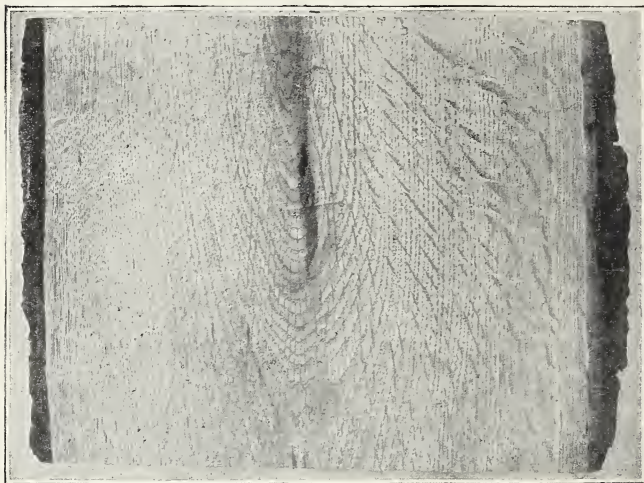
FIG. 22.—Slab sawed lengthwise from a Black Oak. Milford, Pa. The saw passed almost through the center of the tree, but not quite. The lines of annual growth are cut through obliquely, and the silver grain appears quite plainly, both in the middle and at the sides.
