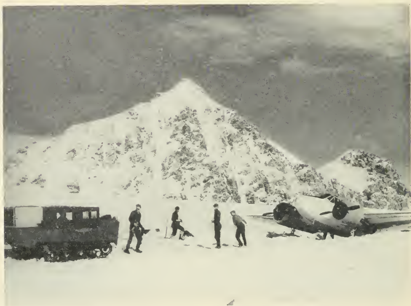
1. WEASEL HAULING THE BEEHCRAFT INTO POSITION FOR FLIGHT AT THE MAIN BASE
