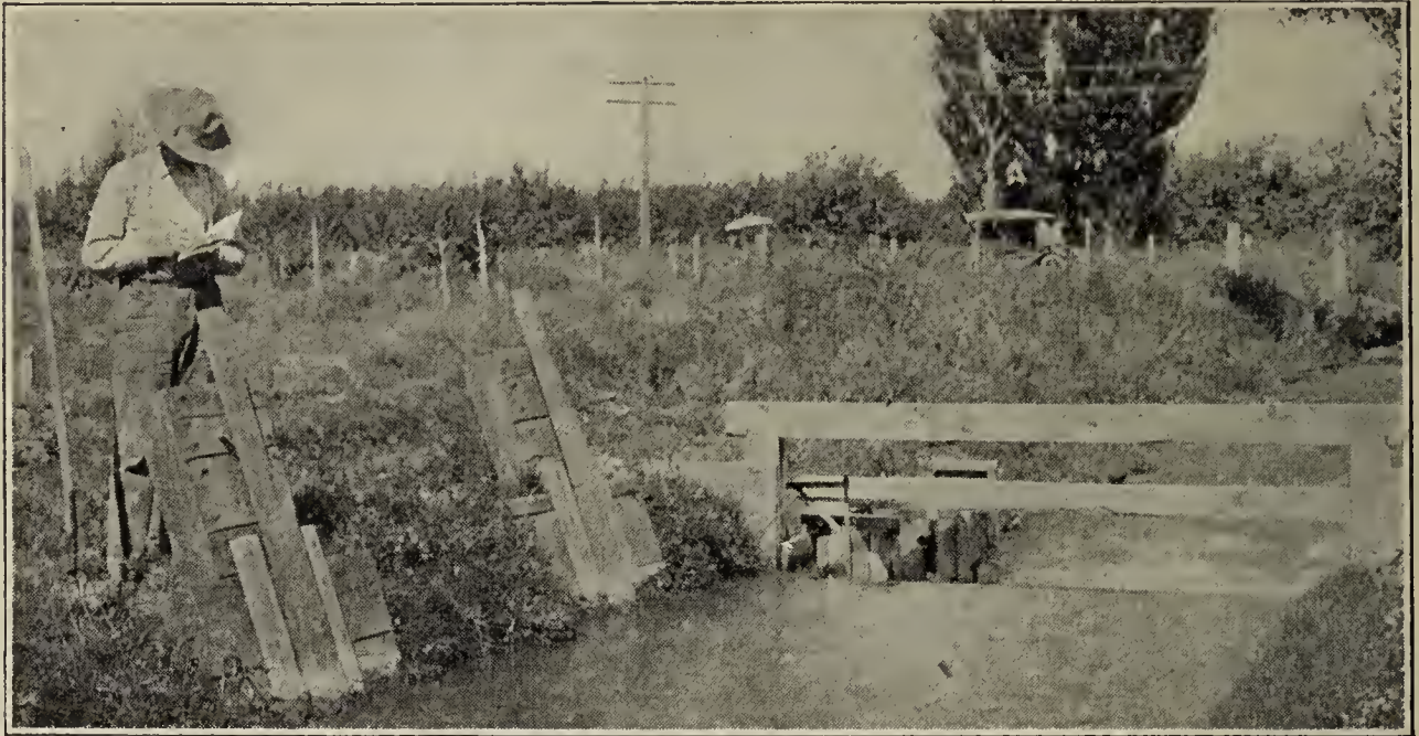
Figure 1. (a) Showing the usual method of placing an Uncompahgre orifice box in a ditch.
