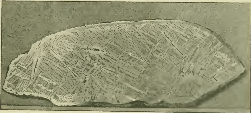
FIG. 2. Section showing Widmanstätten figures (three-fifths actual size).
