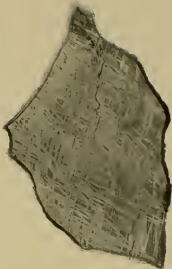
FIG. 3. SECTION SHOWING WIDMANSTÄTTEN FIGURES. (Three-fifths actual size.)
