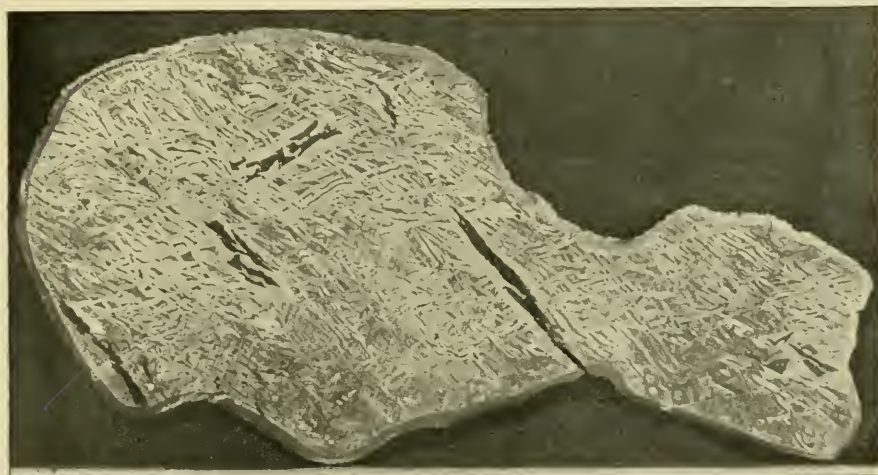
FIG. 3. BALD EAGLE METEORITE. Section showing Widmanstätten figures. Three-fifths actual size.
