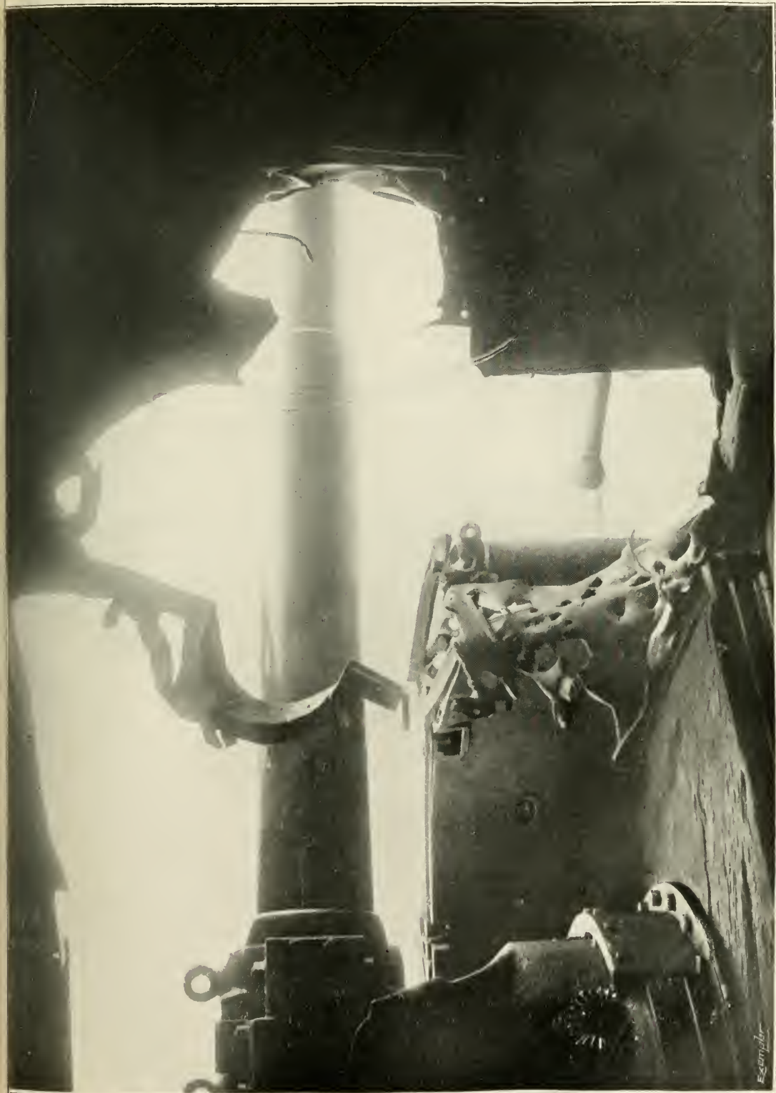
DETAILS OF DAMAGE TO THE FORWARD 8 in. GUN ON THE PORT SIDE ON BOARD THE "ROSSIA." The half-ports and port were shattered by two successive shells which burst in the casemate and caused a fire. The entire gun crew were killed.
