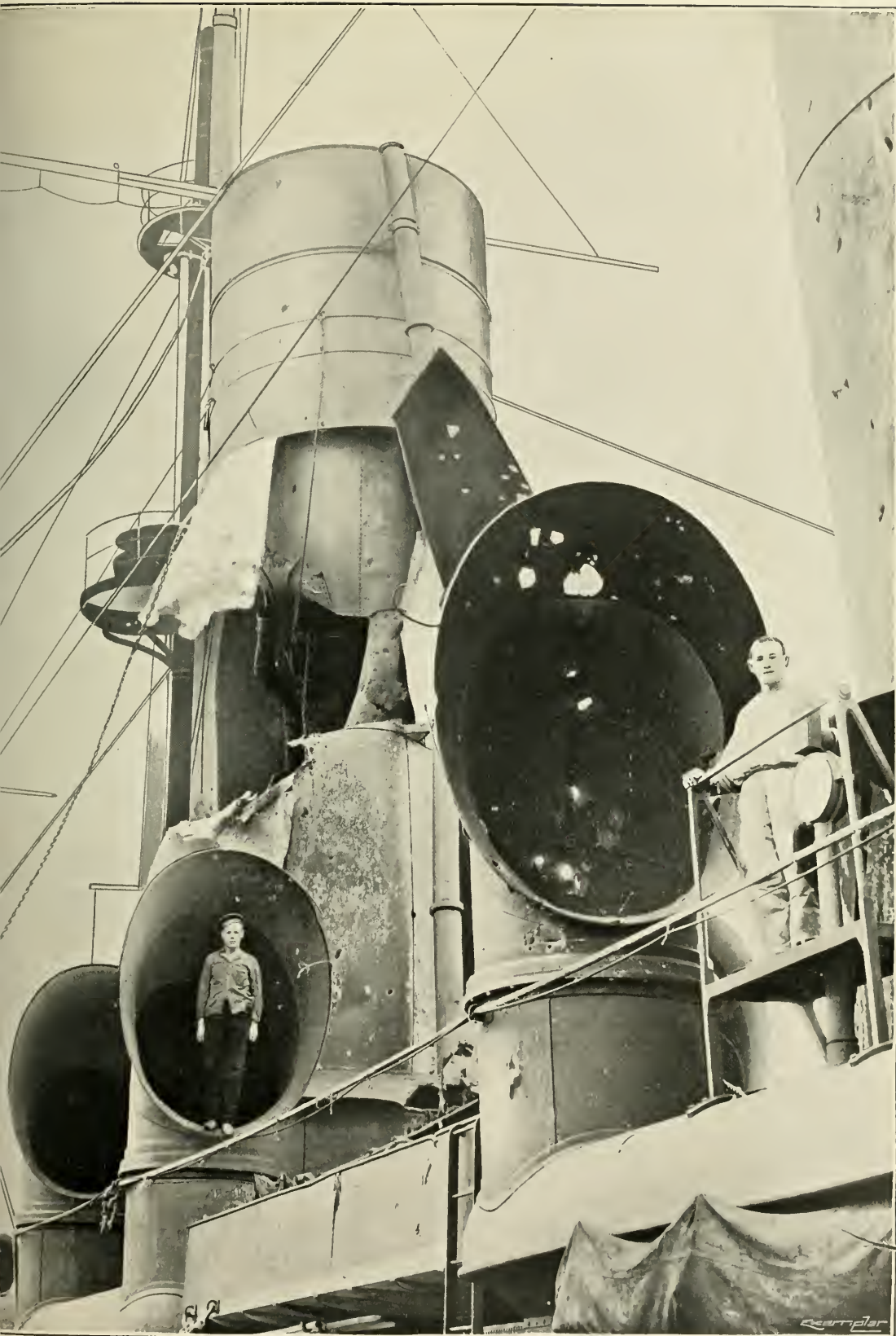
R (FOURTH) FUNNEL OF THE "ROSSIA," CAUSED BY A SHELL STRIKING ON THE PORT SIDE AND EXPLODING INSIDE THE FUNNEL.
