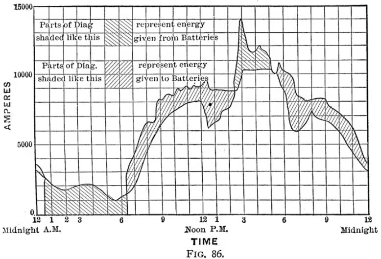
Edison station — for a day in May, 1897, when, because of a sudden storm, the load was thrown on very quickly, the peak of the load being higher than usual. It should also be noted that in case of a breakdown, the battery is ready to carry the entire load for the short time necessary to start up another unit. This is an advantage which will not appeal so much to an outsider, perhaps, as to a man intimately acquainted with station management.
