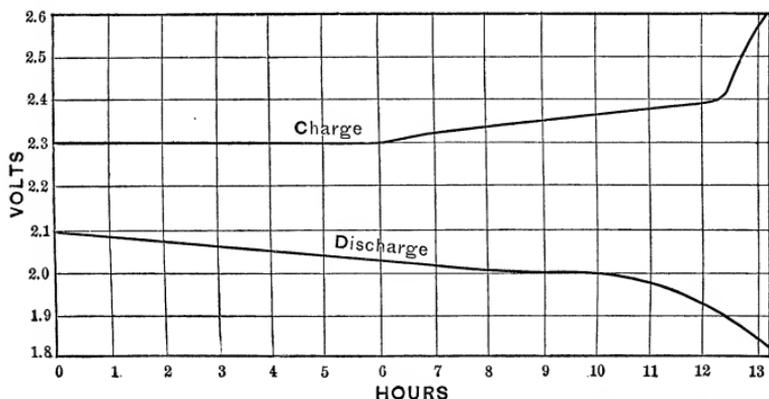
Discharge Curve of Bradbury-Stone Battery. Class B 2, (3).
