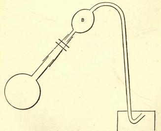
The gases in water are estimated by taking a known volume of water, boiling out the gases, and collecting them
