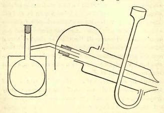
the hot oil or spermaceti, and either the oil-bath may be lowered down away from the flask, or else the flask, which is to be maintained in firm connection with the Liebig's condenser, may be raised out of the oil.
