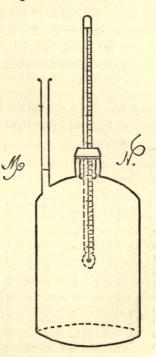
As has been mentioned, I recommend the employment of a half-litre specific gravity bottle; and the weighings are made in my laboratory on a large Oertling balance, capable of carrying a kilogramme, and indicating about a milligramme when heavily loaded.
