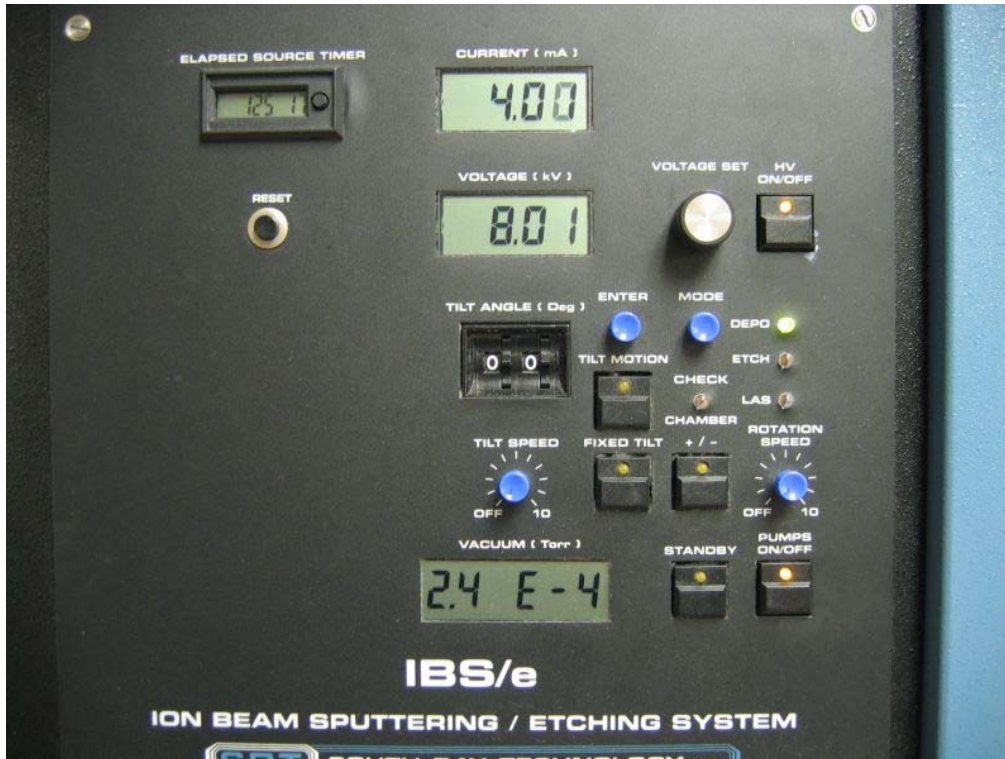
Figure A-4. IBS Control Panel.
