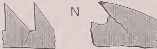
CRACKS FROM ANGULAR FILING.
