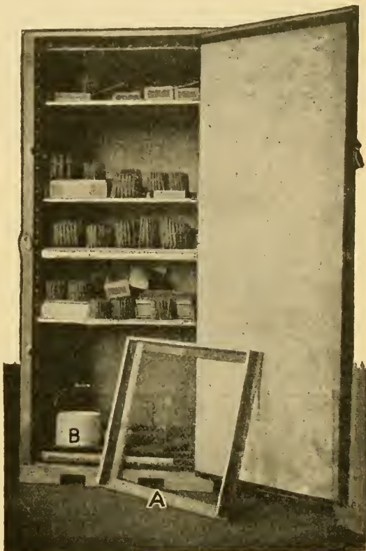
FIG. 16.—A closet for fumigating cigars or manufactured tobacco. A, Removable tray for holding cigars; B, generating jar.
