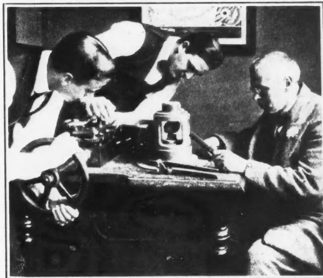
Fig. 3—Splitting a large carbonado
