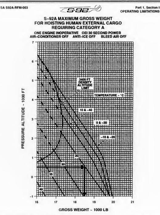
NOTE 1: THIS CHART DEPICTS THE GROSS WEIGHT, PRESSURE ALTITUDE, TEMPERATURE COMBINATION WHERE OEI HOGE CAPABILITY EXISTS USING 30 SECOND OEI POWER WITH A 60 SHP MARGIN.
