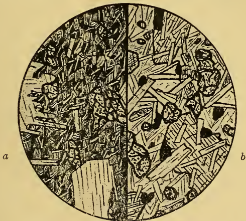
FIG. 3a.—Olivine-tholeiite (Largs type), N.N.W. dyke, shore \frac{3}{4} mile south of Pier, Largs, Ayrshire. \times 20 . Phenocrysts of anorthite and olivine; groundmass: laths of labradorite, grains of augite and olivine, in scanty base of dark glass. \times 20 .
