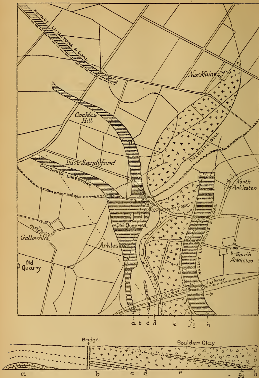
FIG. 2.—Sketch-map and section along the railway at Arkleston, Paisley. a , Blackbyre Limestone with Gallowhill Limestone phase at top; b , Cementstone with rootlets; c , Entomostracan Limestone; d , shales and fireclay; e , dolerite sill; f , Hurlet coal; g , alum shale; h , Hurlet Limestone.
