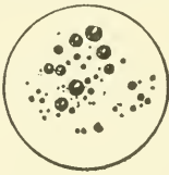
Fig. 1.—Spherical cavities in artificial ruby as seen at one time (enlarged 75 diameters).
