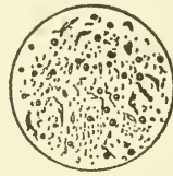
Fig. 2.—Spherical and irregular cavities in artificial ruby as seen at one time, evidently from the lower part of the crucible (enlarged 25 diameters).
