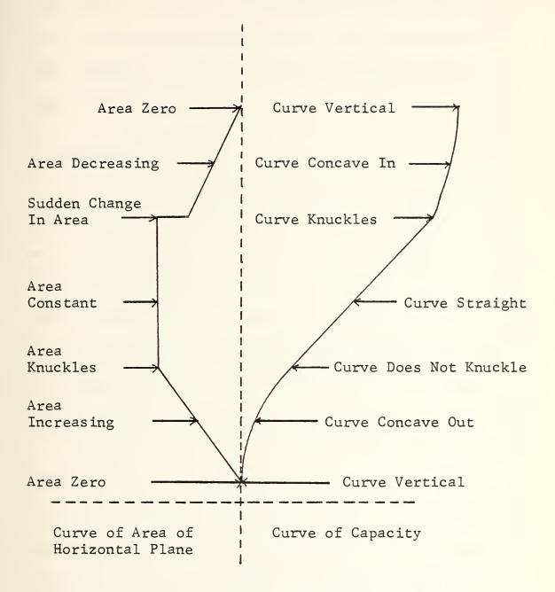
Figure 5. Tank Shape vs. Capacity Curve Shape
