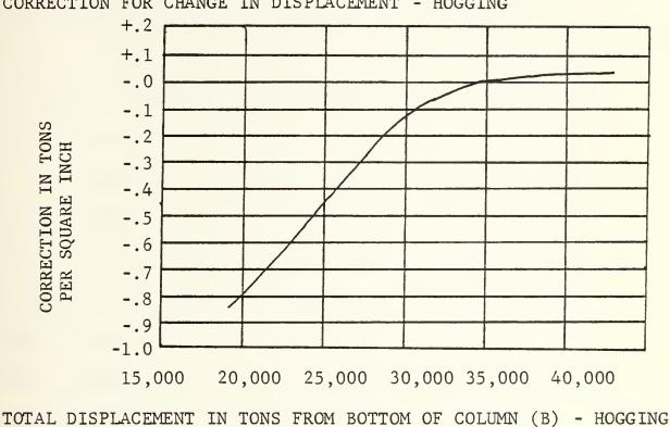
CORRECTION FOR CHANGE IN DISPLACEMENT - HOGGING
