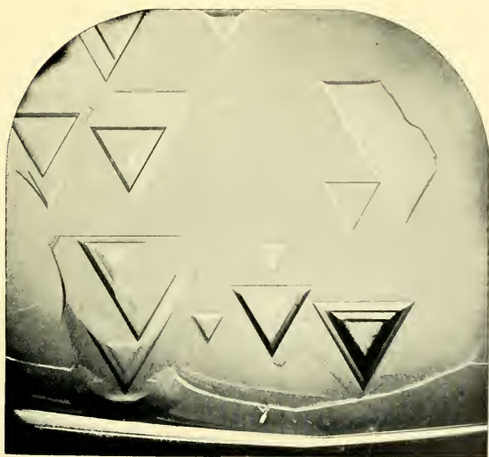
22.—Triangular Markings on a Crystal of Diamond ( \times 100 ).
