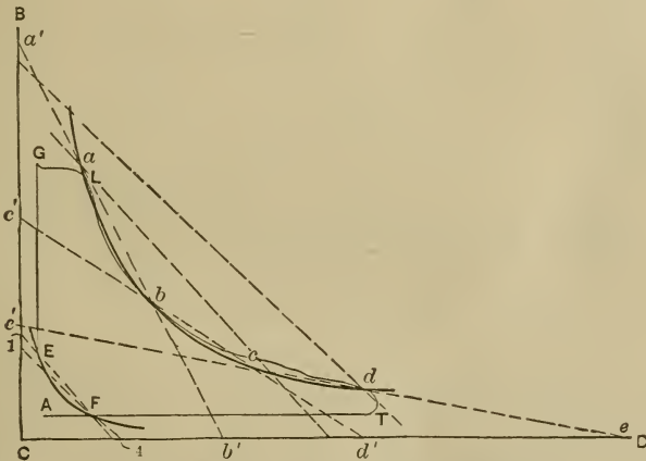
FIG. 45.—Method of Drawing an Hyperbola.
