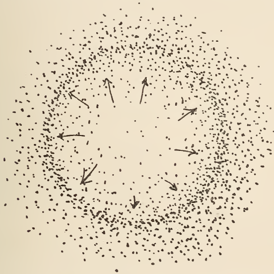
FIG. 13. Migration of Silver Particles in Water Spot.
