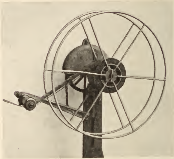
FIG. 2. Front View of Rewind (Dummy) Showing Reel Catch Finger.
