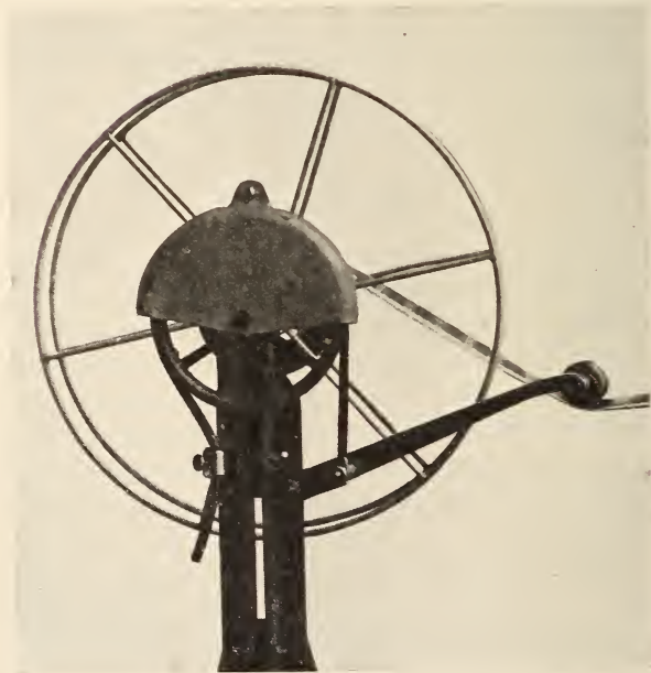
FIG. 3. Rear View of Rewind (Dummy) Showing Automatic Brake.
