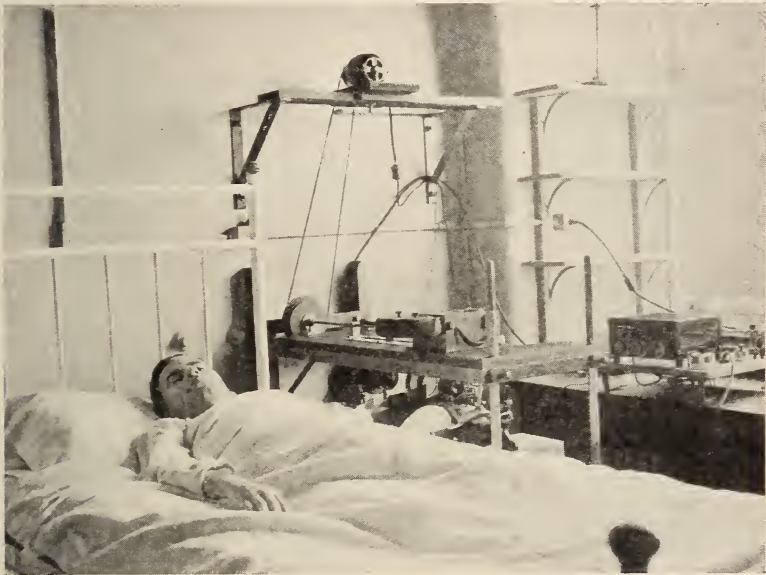
FIG. 7—Apparatus for taking motion pictures of human capillaries (capillarograph).
