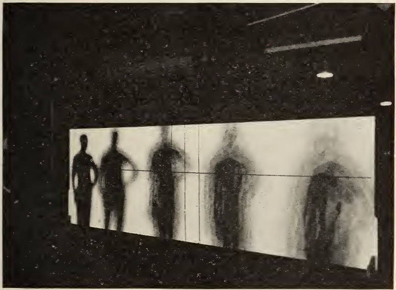
Fig. 5—A study of the shadows formed by a polygonal mirror. There is a separate shadow for each section of the polygon, 16 in this particular case.
