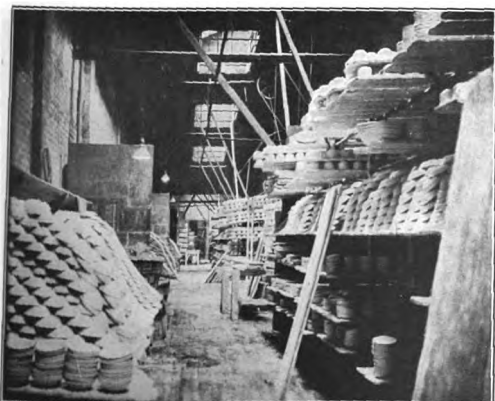
FIG. 32.—DIPPING ROOM. NOTE NARROW AISLE AND GLAZE-COVERED FLOOR.
