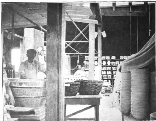
FIG. 19.—SHOWING DRYING RACKS, AND WARE AND DIPPING TUB IN A LARGE ROOM.
