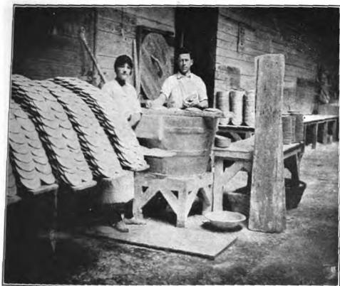
FIG. 31.—DIPPING. NOTE GLAZE ON FOREARMS OF THE DIPPER. HANDS OF DIPPERS' HELPERS ARE ALSO COVERED FROM HANDLING THE WET DIPPED WARE.
