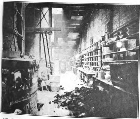
FIG. 21.—KILN ROOM SHOWING WORK BENCHES (ON RIGHT) WITH WARE BOARDS AND WARE ON SUPPORTS, KILNS ON LEFT, COAL ON FLOOR IN FOREGROUND, AND GENERAL UNTIDY CONDITION OF KILN ROOM.
