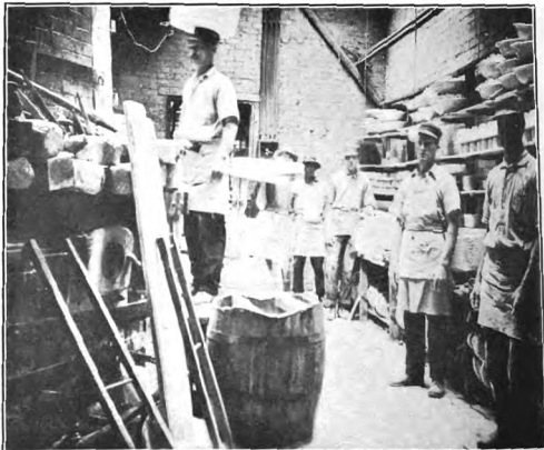
FIG. 27.—KILN PLACING. NOTE KILN PLACER WITH LOADED SAGGER ON HEAD CLIMBING STEPS OF KILN, WARE BOARDS LEANING AGAINST KILN, WARE CARRIER OR KILN PLACER IN BACKGROUND WITH WARE BOARD COVERED WITH DIPPED WARE, KILN PLACERS OR SAGGER LOADERS AT WORK BENCHES, WARE BOARDS WITH WARE ON BRACKETS ABOVE WORK BENCHES, APRONS ON WORKMEN, CLOTHING OF WORKMEN AND CONDITION OF FLOOR.
