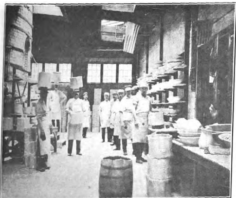
FIG. 17.—GLOST KILN PLACING. NOTE MEN WITH SAGGERS ON THEIR HEADS, STEPS LEADING INTO KILN, WORK-BENCHES, POTTERY WARE, WORK APRONS, AND ILLUMINATION OF ROOM. THIS ROOM IS WELL LIGHTED.
