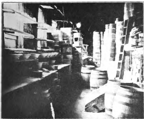
FIG. 29.—WORK BENCH IN GLOST KILN ROOM. NOTE CONGESTION AND POOR ILLUMINATION.
