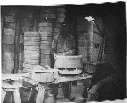
FIG. 14.—SAGGER WASHING. NOTE GLAZE ON HANDS OF WORKER AND DRY GLAZE ON EQUIPMENT.
