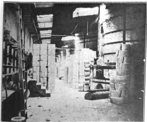
FIG. 16.—GENERAL VIEW OF A GLOST-KILN ROOM, SHOWING SAGGERS WARE WORK BENCHES, KILNS, AND ROOF ILLUMINATION.
