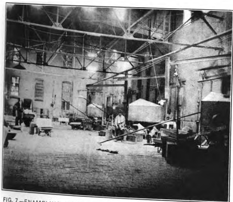
FIG. 7.—ENAMELING ROOM. NOTE GOOD NATURAL ILLUMINATION AND POSITION OF LOCAL LAMPS.
