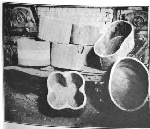
FIG. 2.—DIFFERENT TYPES OF SAGGERS.
