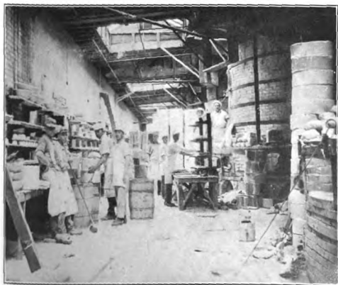
FIG. 30.—KILN PLACING ROOM AND WORK BENCH. NOTE GOOD NATURAL ILLUMINATION AND ABSENCE OF CONGESTION.
