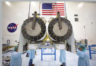
NASA and Boeing workers help position the first two of six ISS Roll-Out Solar Arrays (iROSA) onto flight support equipment inside the high bay of the Space Station Processing Facility at Kennedy Space Center. This pair was launched on CRS-22.
