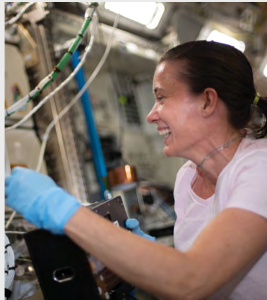
NASA astronaut and Expedition 65 Flight Engineer Megan McArthur removes Kidney Cells-02 hardware inside the Space Automated Bioproduct Laboratory and swaps media inside the Microgravity Science Glovebox. The human research study seeks to improve treatments for kidney stones and osteoporosis.
