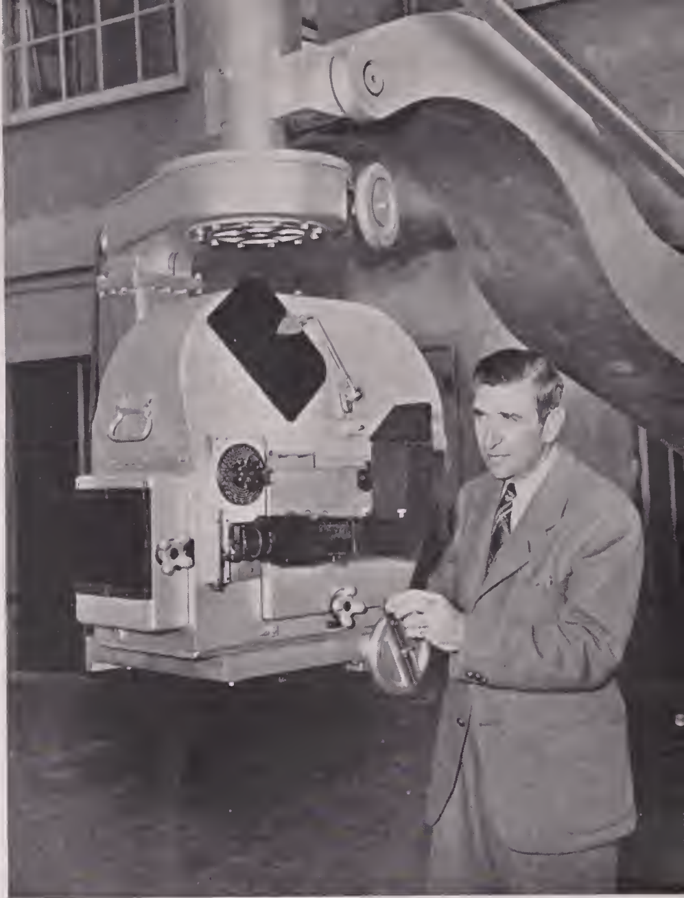
Camera Chief Arnold operates the quick-action pan on his new camera carriage. Note underslung camera mounting and inverted periscope on finder. Fourteen turns of the wheel under Arnold's hand pans camera through full circle; tilt also permits full-circle rotation.
