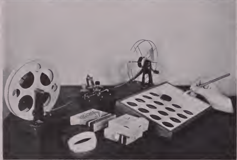
For systematic editing, this rack has film strip holes for temporary storage during cutting. Description of each scene is written on film record pad at right opposite proper hole number.
