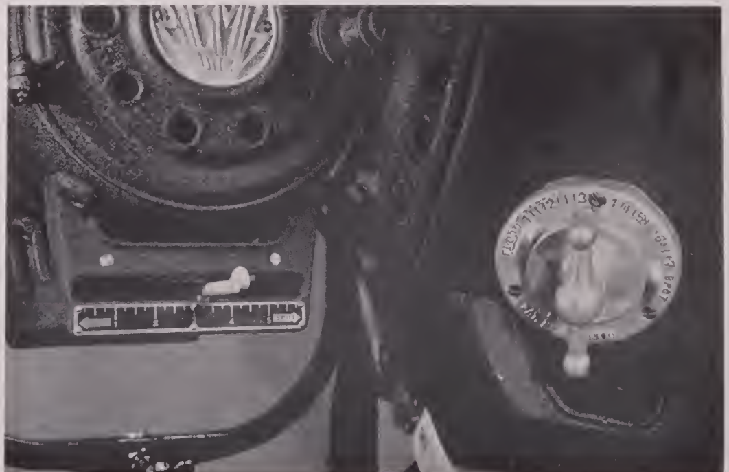
Left, closeup B-M quick focusing device for Baby Keg-Lite. Right, closeup B-M quick focusing device for 2000-watt spot.
