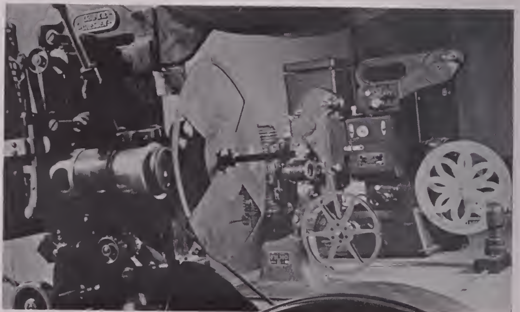
Fifteen years of projector progress—35mm., 8mm. and 16mm. Note lenses are at approximately same height for uniformly good projection; little tilting is necessary.
