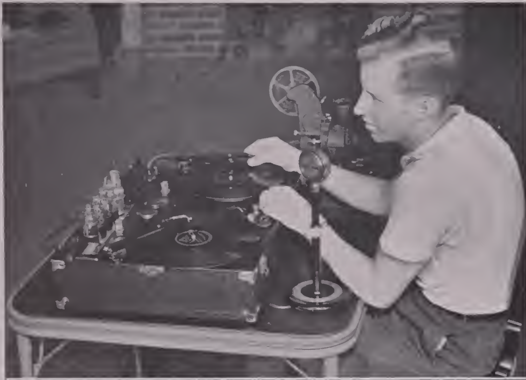
George Culbertson of the Minneapolis Cine Club is shown with his deluxe dual turntable outfit, which he built for sound synchronizing amateur-made movies.
