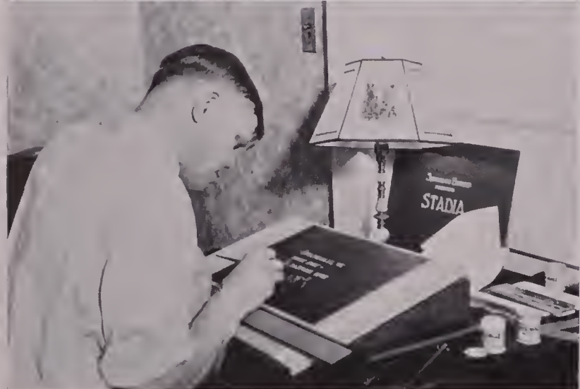
Lettering white-on-black title cards for reversal filming. For wobbly printers, special lettering guides and tracing alphabets are available.
