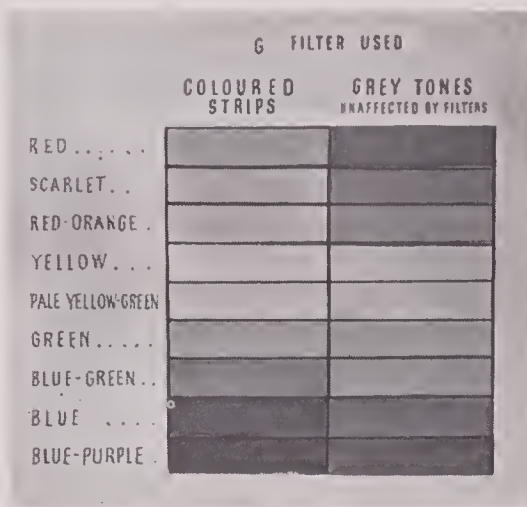
G. FILTER. An orange filter which produces over correction, absorbs the blue light which is prevalent in shadows on a clear day, thereby making them appear darker. It will remove haze and atmosphere from a scene, but should not be used on a sea-scape unless it is required to make the water appear almost black.
