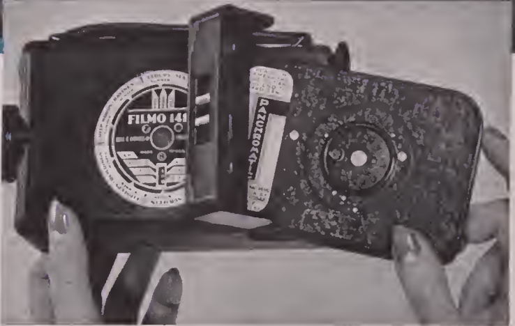
NO THREADING OF FILM —Just open the door, slide in pre-threaded magazine of 16 mm. color or black-and-white film, snap door shut, and Filmo 141 is loaded, ready to take the kind of movies you've always wanted—clear, sharp pictures true to color, true to life!
