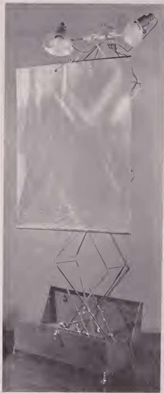
Agfalite set up, with distance between lights varying from 11 to 36 inches and elevation at any point up to 94 inches.
