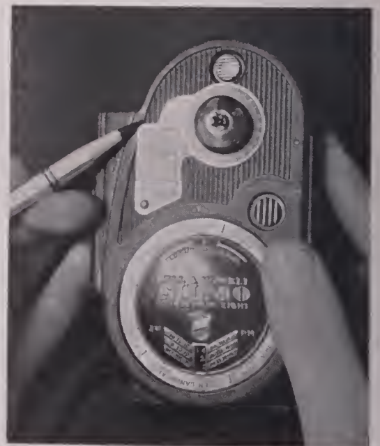
Outside of movie camera cover shows wind-back knob and calibrations to insure accuracy. Number of turns per foot depends on size of loaded film spool. Arbitrary A to Z letters aid in marking rewind position.
