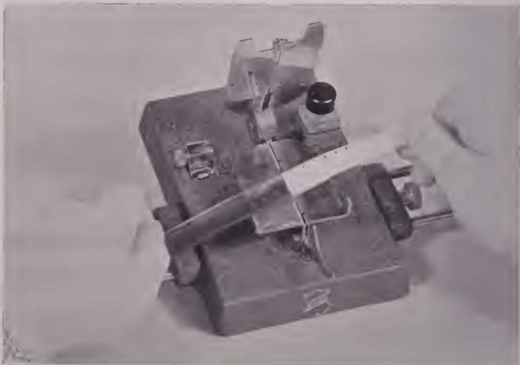
Filmo 16mm. film splicer showing diagonal splice. Lugs fitting into perforation hold at proper angle.
