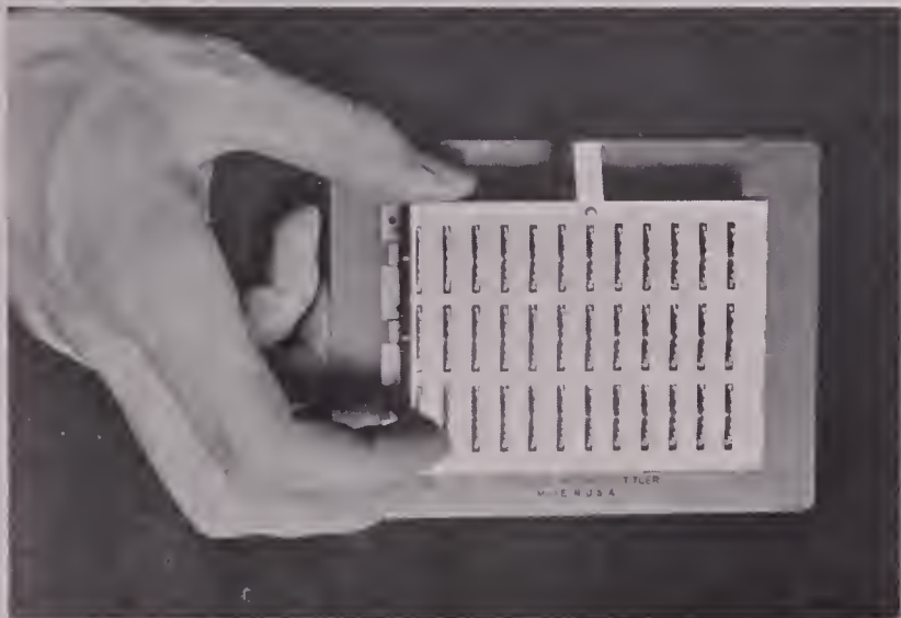
Rear of the new title-builder showing three rows of 12 wheels, each of which operates continuous ribbon on which 42 characters are imprinted.
