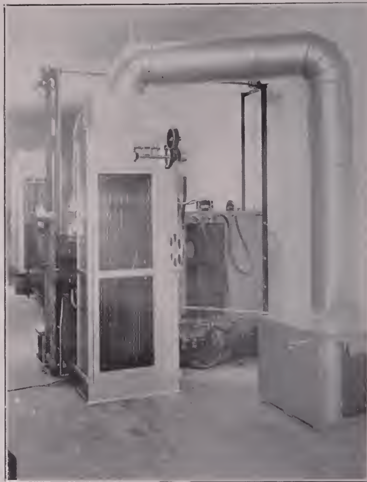
Front view of 16mm. developer showing dry box and blower equipment
