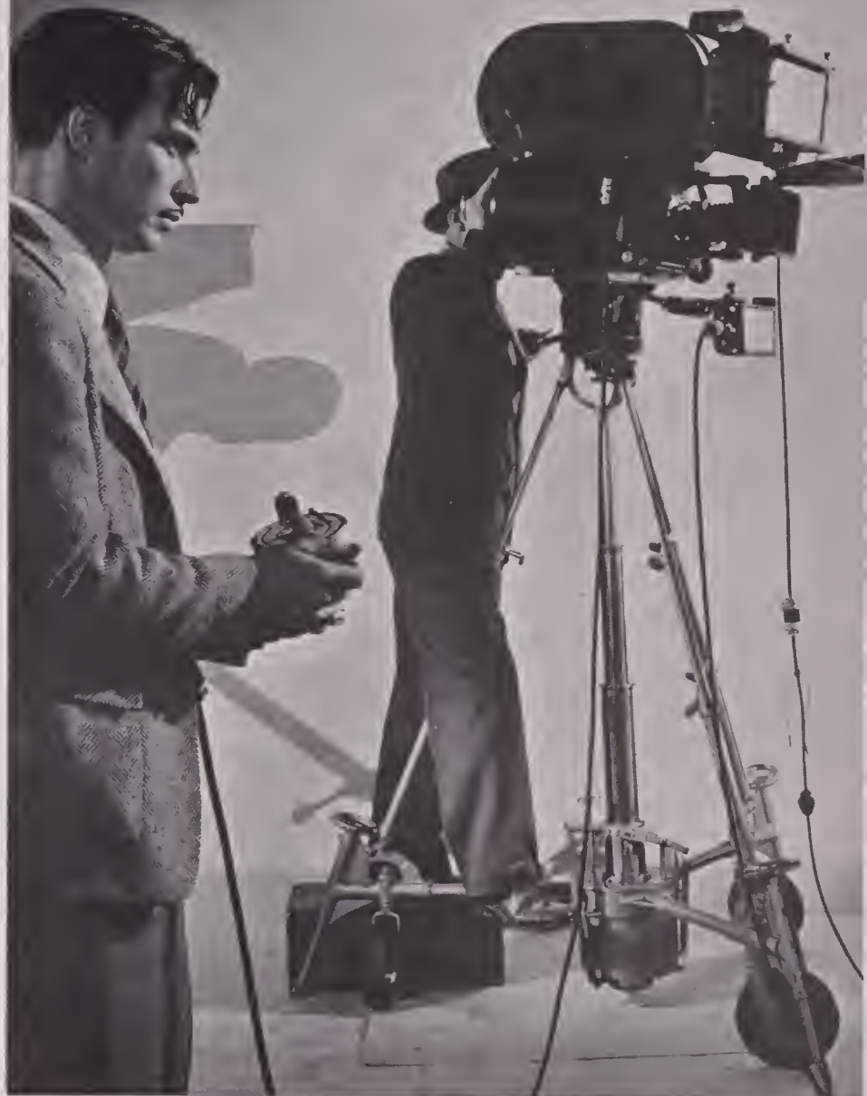
Toland's outfit at work. Note "filler" lights on front of camera, hydraulic-hoist rolling tripod, and remote-control focusing dial in hands of Assistant Edward Garvin, left foreground.
