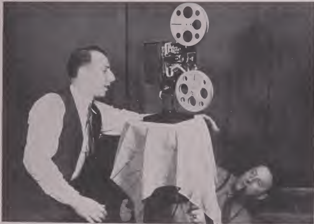
To swing projector for smooth right angle turn for title background, machine was set atop swivel chair. Ray Rieschl (left) assists, while Edward Johnson, sprawled on floor, does manual labor.
