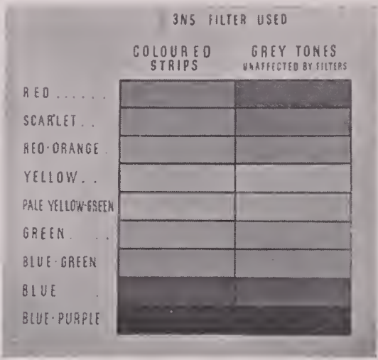
3 N. 5. This filter is a combination of an aero 1 and a neutral density filter. It does not give over correction but is capable of producing highest pictorial qualities on either pan or super pan film. This filter can be thoroughly recommended to the amateur.
