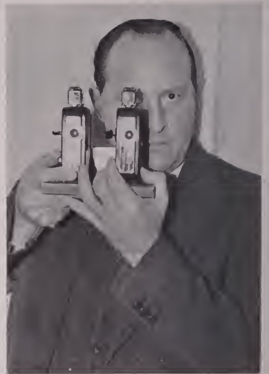
Dr. Ghrist demonstrates his 8mm stereo cameras. The two machines are kept in synchronization by a shaft in the mounting base with a gear on each end which meshes with gears in the camera motor.
