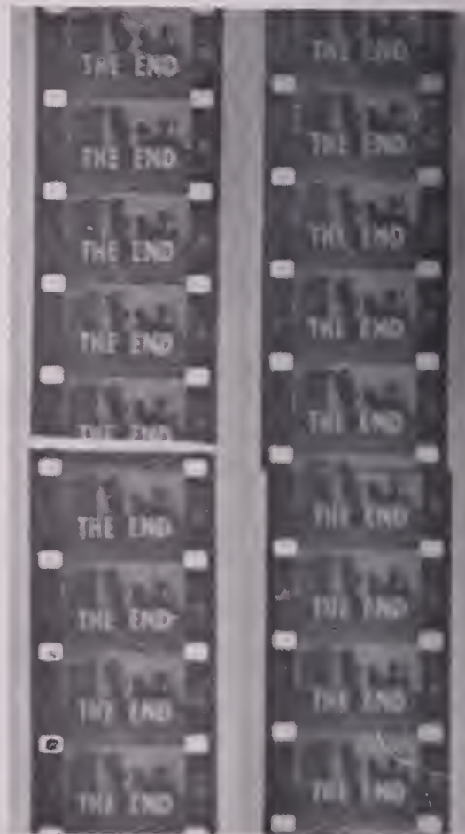
Splices made with a faulty splicer.
