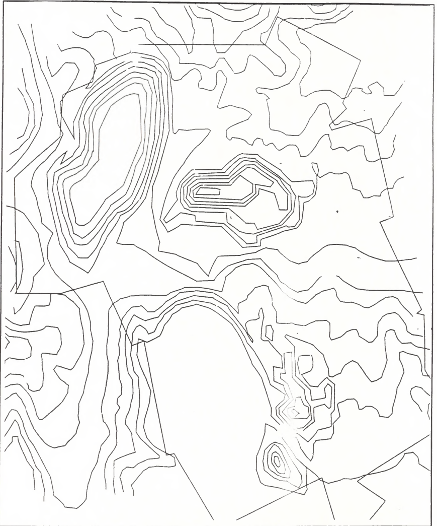
Figure 4: Post-Reclamation Contours of the Baltic Mine Project
