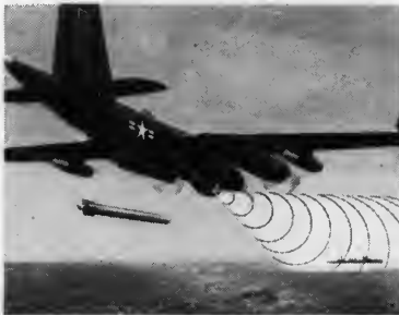
These drawings illustrate the multiple-mission capabilities of the P2V Neptune : 1 Low-flying P2V's electronic gear spots submerged sub because its presence distorts the earth's magnetic field. 2 Depth-bombing a submerged sub, 3 torpedoing a surface ship or laying mines to disrupt enemy shipping are jobs the P2V can do equally well. 4 Spotting hurricanes and reporting their velocity and direction are routine but important P2V missions which save human lives and vast sums in property damage.
