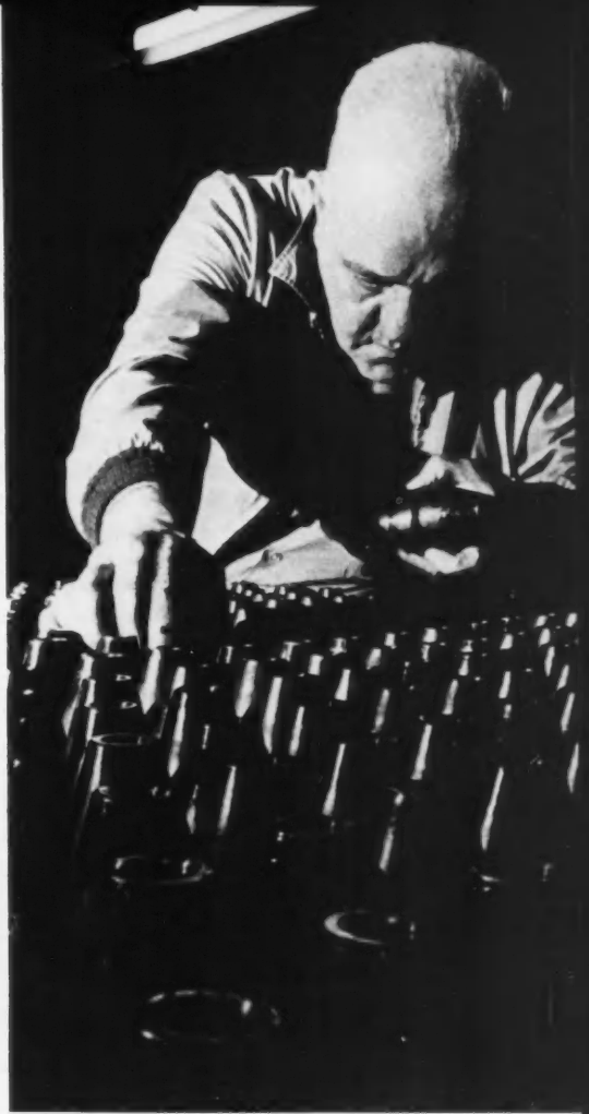
An industrial ammunition inspector makes final check of the casing of 60mm mortar shells prior to painting at an ammunition plant in Danville, Pa. Administering the defense contracts of plants is a major mission of the Defense Supply Agency.
